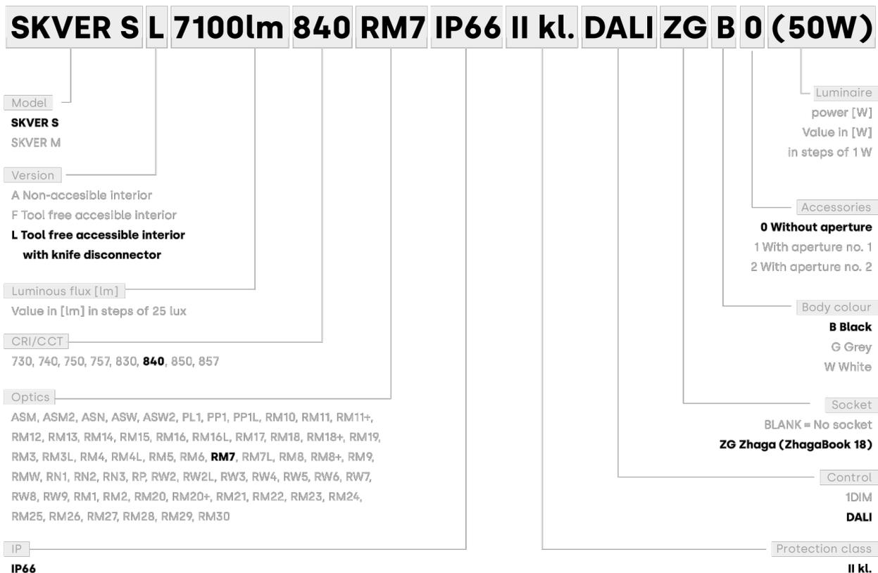
The Skver LED luminaire is available in 6 types:
